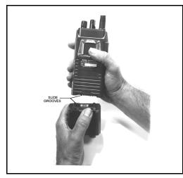
Figure 8 - Installing the Battery Pack
